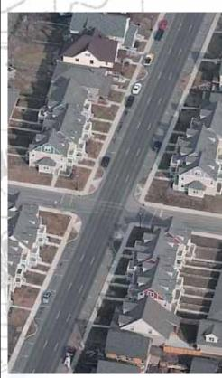
Bump-outs are an excellent way to introduce street trees into a street while not reducing the width of the travel lanes and still accommodating parking needs. Bump-outs usually are placed at intersections, where they narrow the distance of the pedestrian crossing while increasing pedestrian visibility and safety. They are also placed at regular intervals along the street, where they provide space for street trees and/or lights.
